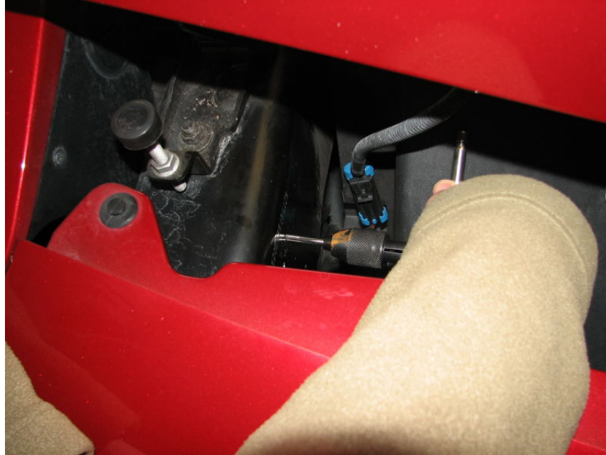
Figure 8: Threading holes with 8-32 tap
