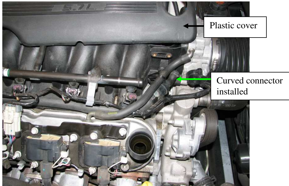
Figure 10: Removing the plastic cover
