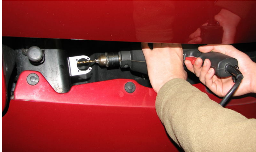
Figure 4: Drilling bracket holes
