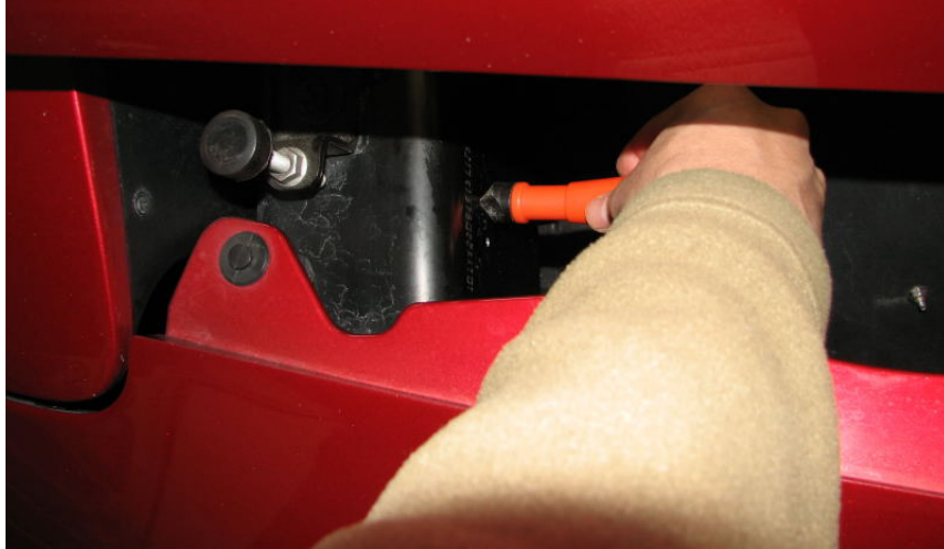
Figure 6: Using the countersink tool
