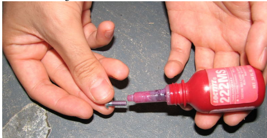
Figure 9: Applying thread-locking compound.
