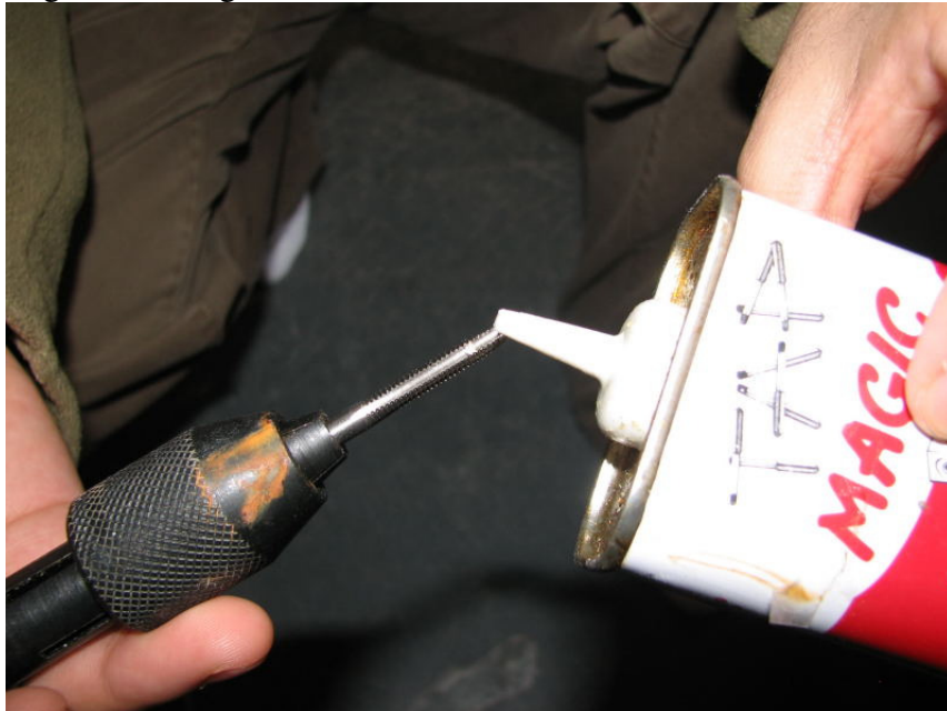
Figure 7: Applying tapping fluid to 8-32 tap
