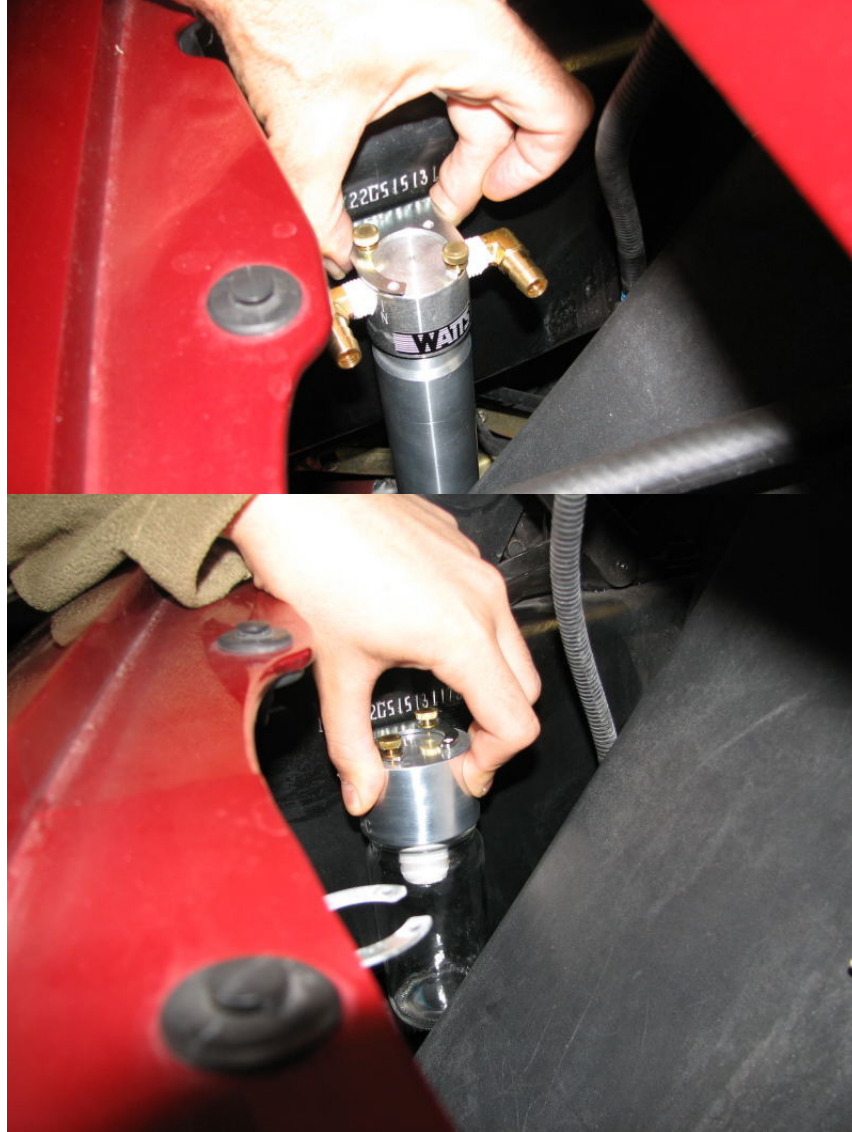
Figures 1 and 2: Catch can mounting position alignment
