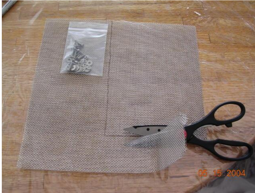
Figure 18: Cutting stainless steel wire mesh
