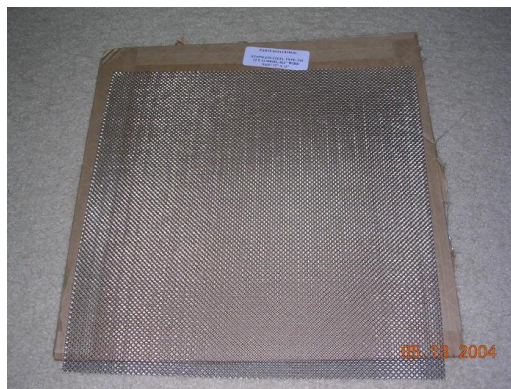
Figure 3 • 12 x 12-inch stainless steel wire mesh, part number 9319T547 (McMaster-Carr, www.mcmaster.com )
