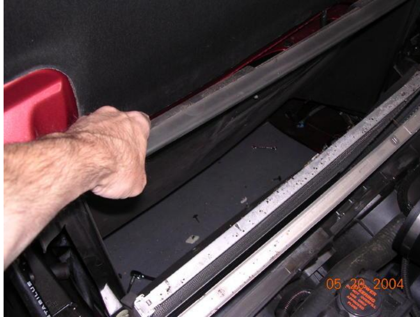
Figure 16: Pulling out radiator cover
