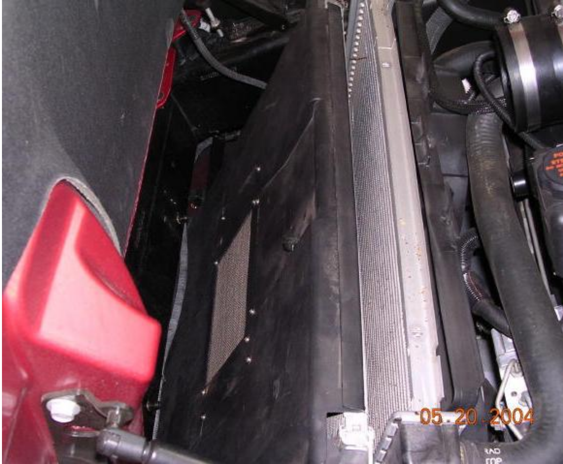
Figure 25: Installed radiator cover
