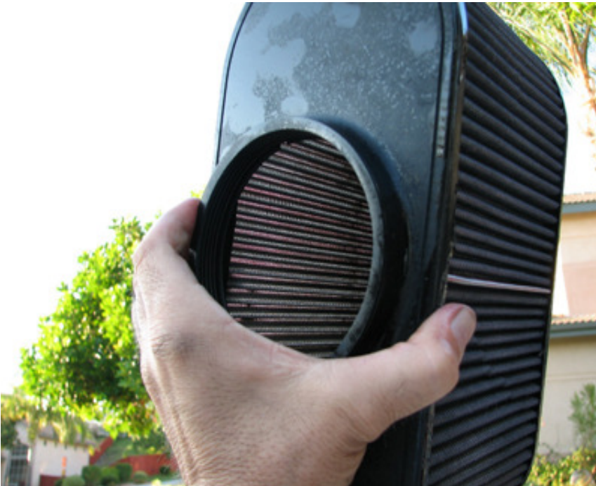
Figure 10: inside of adequately-oiled filter
