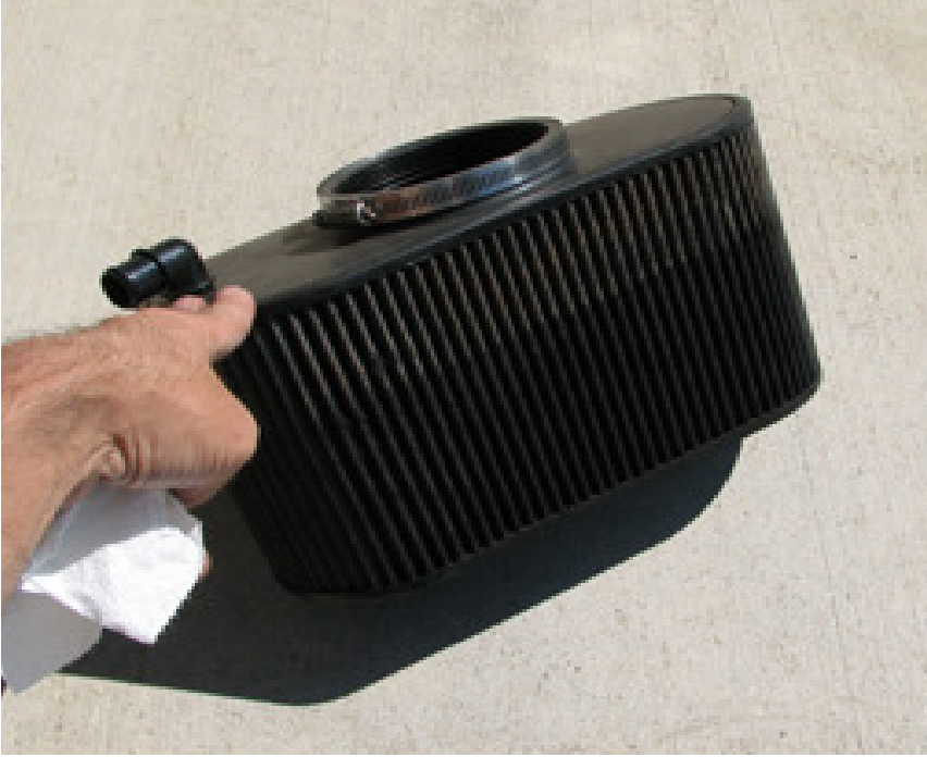
Figure 4: CAI inlet side of filter
