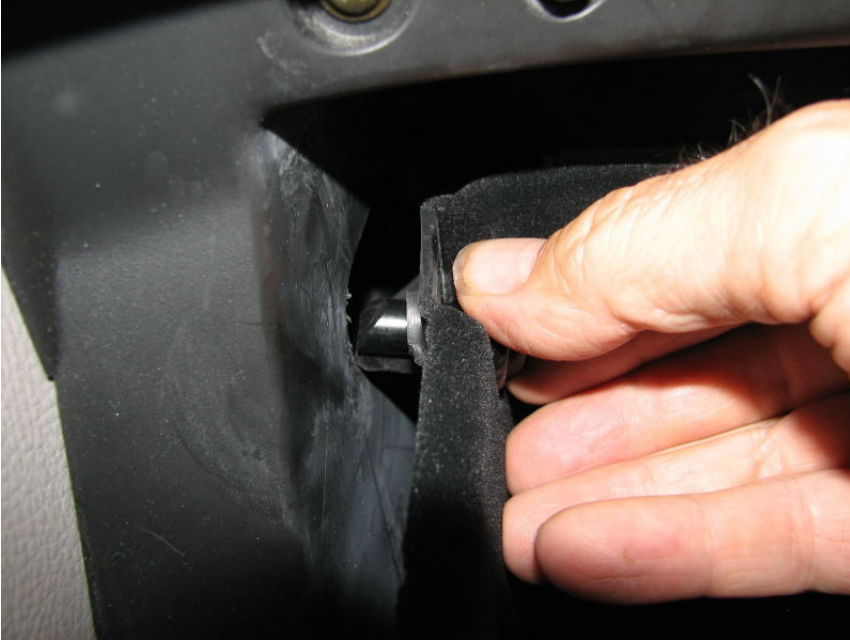
Figure 11: Pulling left side button inward
