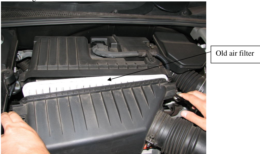
Figure 5: Removing old air filter
