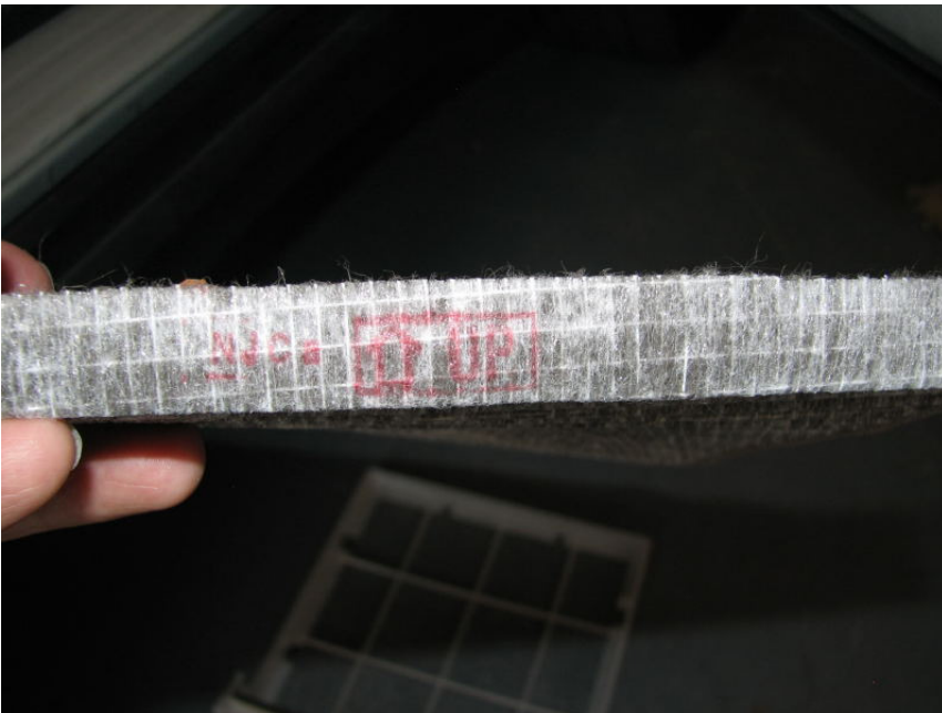
Figure 16 : OEM filter mounting direction indication
